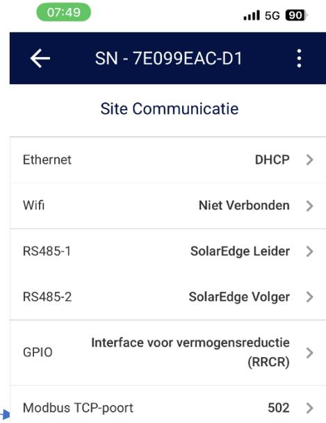
The IP address can be found at monitoring communication within the same menu. This IP address needs to be added in the configuration file.
